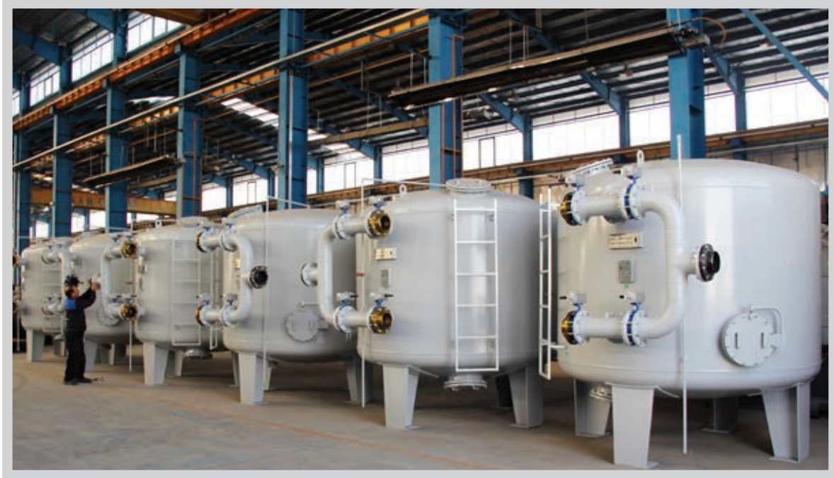
▲ Vertical Sand Filters with pneumatic valves
