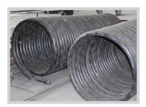
Hot oil boilers are produced in single-coil, dual-coil, or triple-coil types based on their capacities. Each coil is composed of one, two or three tubes next to each other.
